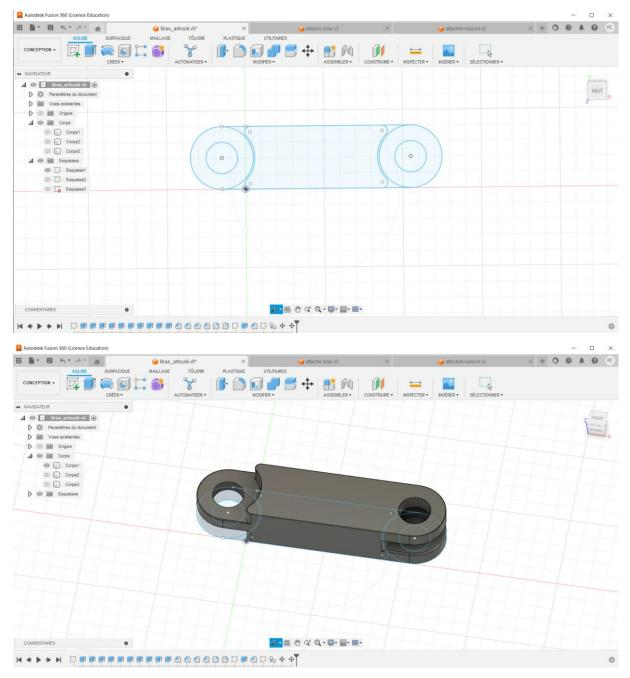
It's important to note that the first part of the arm and the second part of the arm are two identical parts, so that their assembly is as precise as possible. Adding a chamfer makes for better assembly during printing, and also prevents the part from breaking when it's removed from the 3D printer tray.
