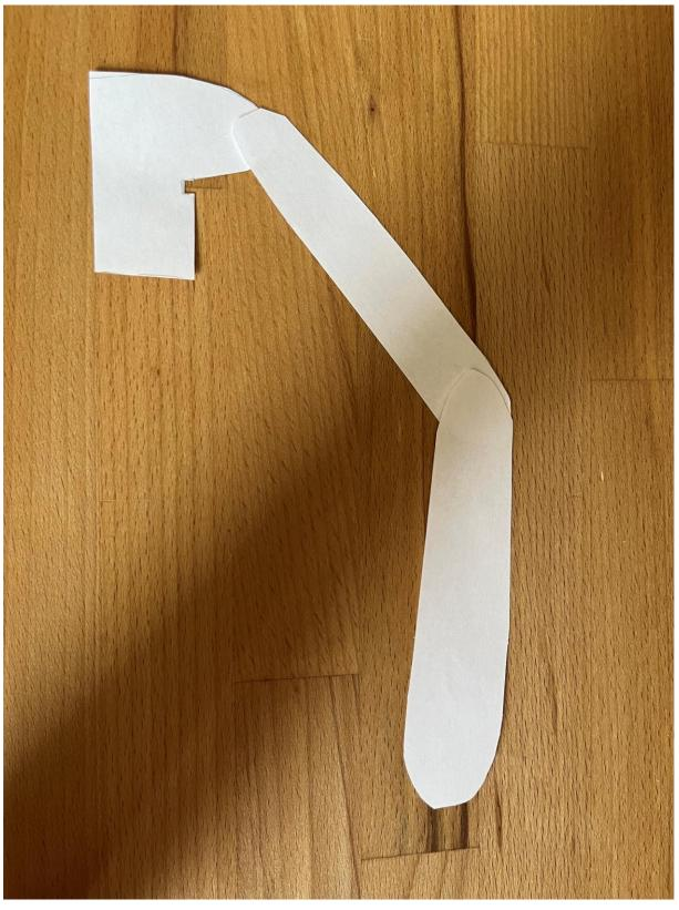
We drew the various parts of our robotic arm in 2D so that we could analyse how well our project worked as imagined in our heads. This is called a cardboard and it allows you to visualise a prototype before printing or manufacturing it for the first time. Thanks to the cardboard, you can see the different constraints that need to be met and avoid encountering them when assembling the first prototype. This method enabled us to highlight a number of points for reflection, such as :
